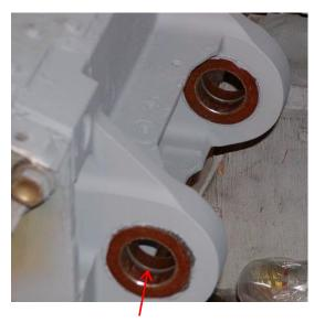
From this configuration with a gap in the middle; *Two* flanged bushings pressed in from either side
