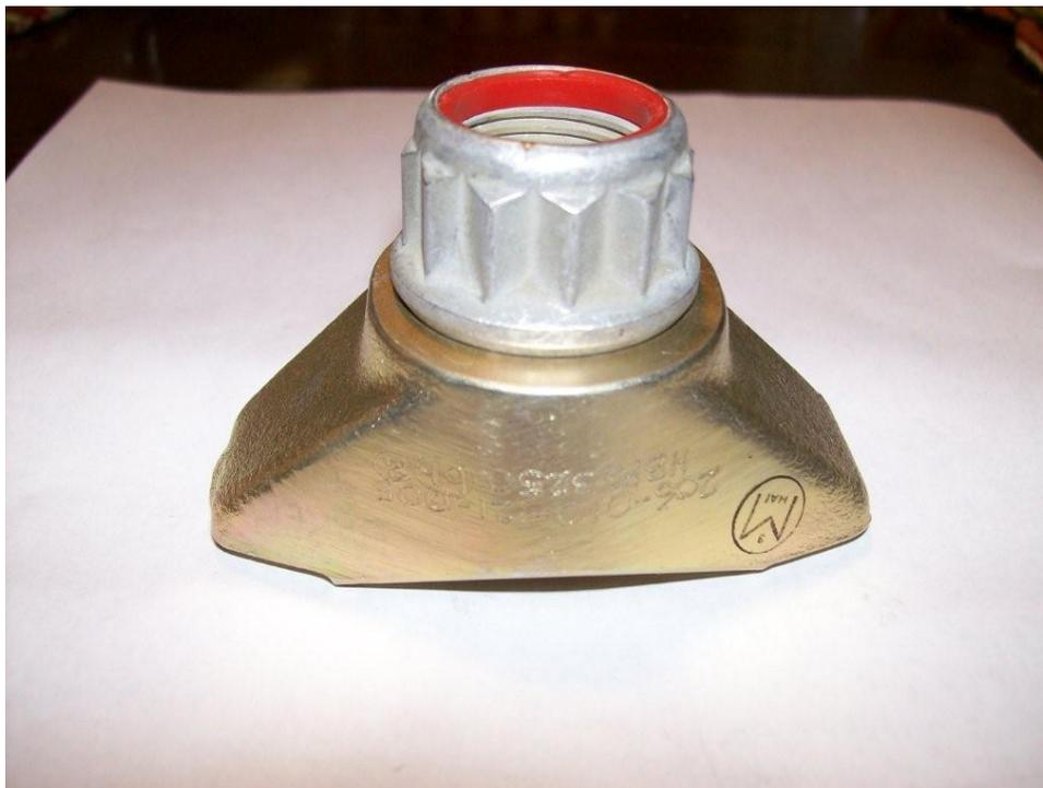
Figure 4: Example Correct Nut as seen with Main Rotor Latch - Note close tolerance fit.
