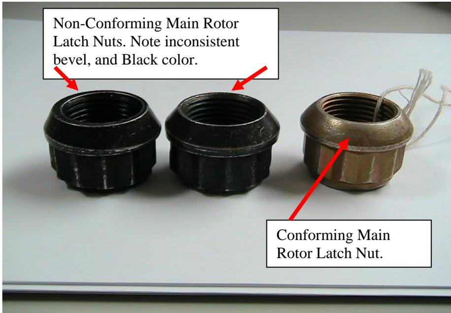
Figure 1: Comparison Non-Conforming MR Nuts with Conforming Nut
