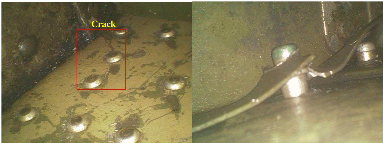
Figure 3, Damaged P/N 206-032-200-21, Thin Bulkhead
