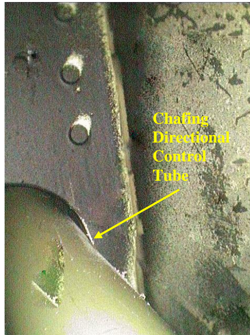
Figure 4, Chafing, P/N 206-001-020-33, Connecting Link
