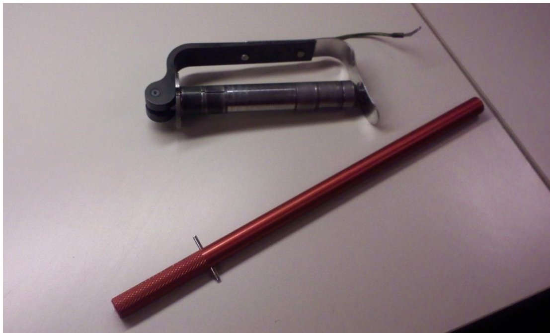
Figure 2: MR Blade Pin Cleaning Tool, NSN 5120-01-475-9901, PN 156058DBPCT, and MR Expandable Bolt, PN 406-310-103-101
