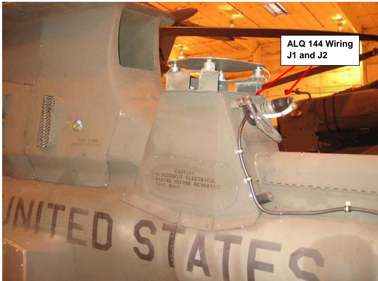
FIG 1: AN/ALQ-144 Countermeasures Set J1 and J2 Cables secured to "Dummy" receptacles.
