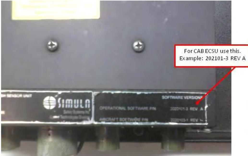
Figure 7: CABS ECSU Software Identification label REV A
