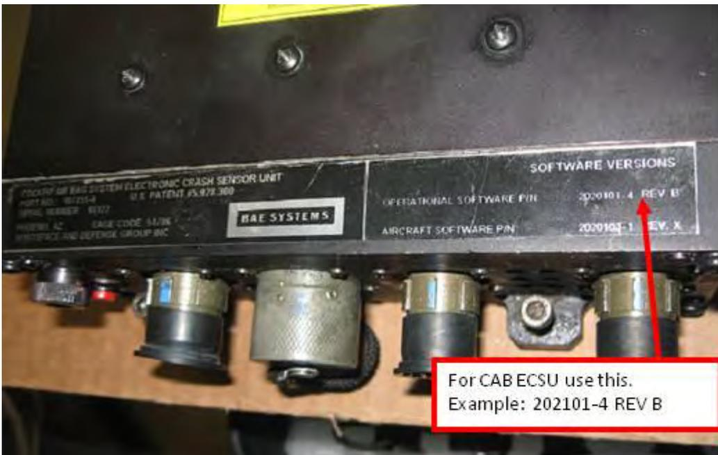
Figure 8: CABS ECSU Software Identification label REV B
