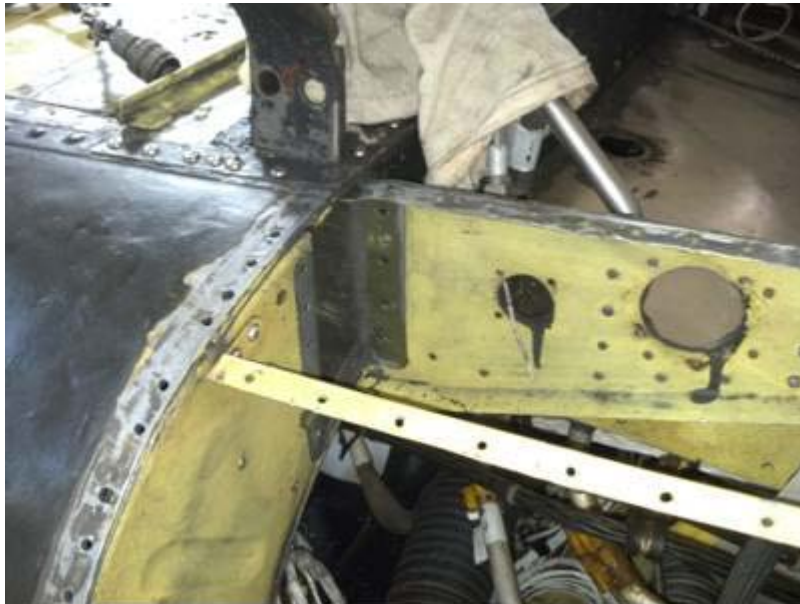
Figure 2: Inspect for cracks along edge of angle and at rivet locations
