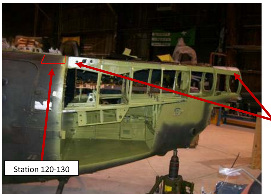
Figure 4: Left side cut away showing longeron from Station 130 bulkhead to tailboom fitting.
