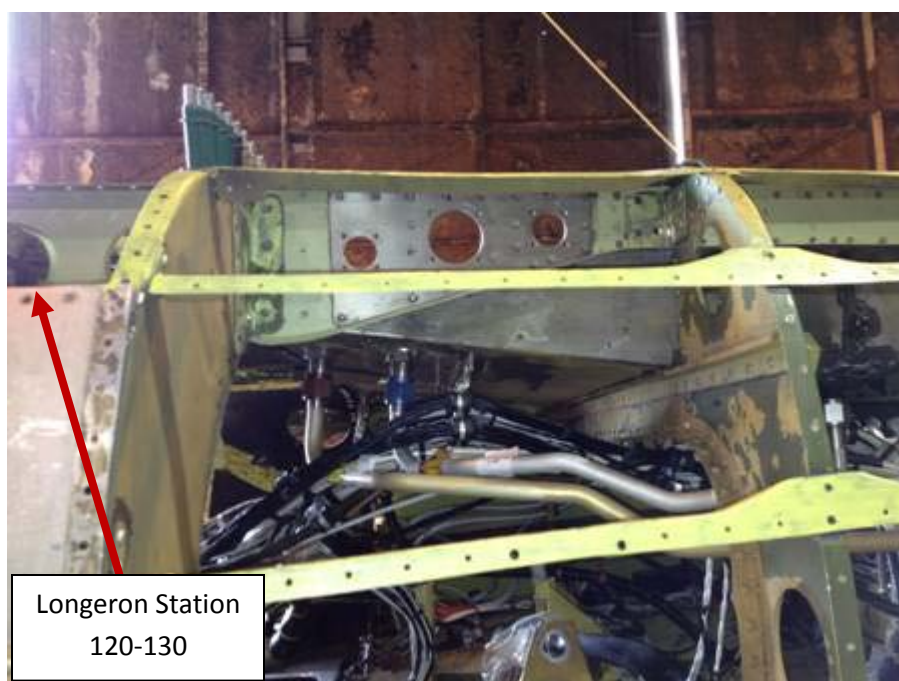
Figure 5: Cutaway left side longeron at FS 130 bulkhead Longeron Inspection Right Side (PN 206-031-314-55)
