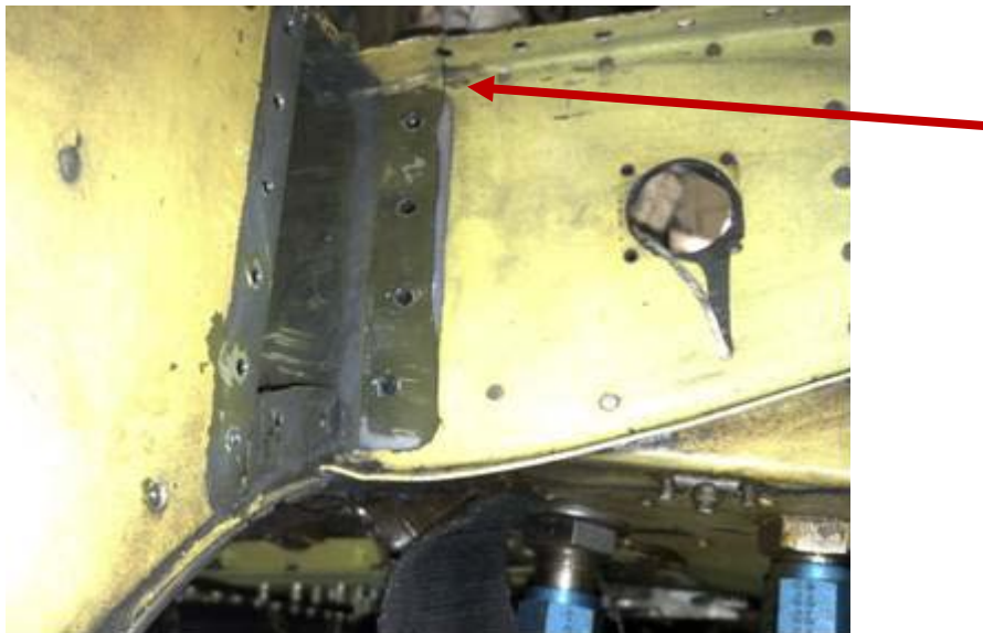
Figure 3: Example crack at fastener location, angle removed.
