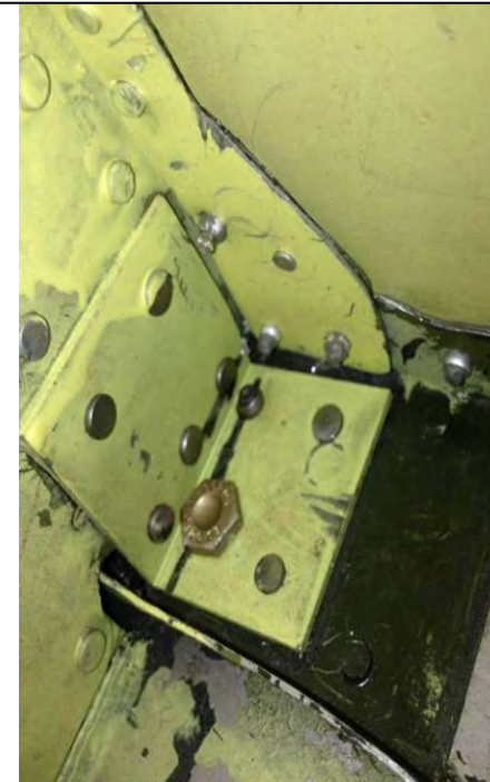
Non-Conforming: No Fillet Radius OR Bell Helicopter (bh) Stamp (recent install)
