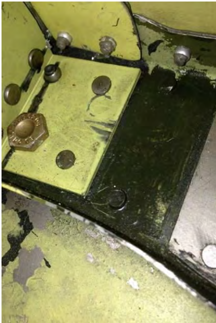
Non-Conforming: No Fillet Radius, 90 Degree sharp edge
